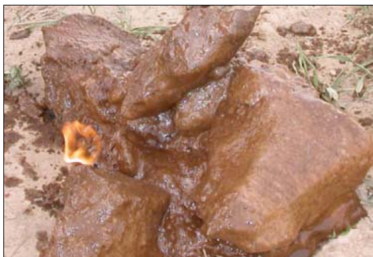
The object's flammable nature suggested hydrocarbon content, helping confirm hydrate formation in the pipeline (Fig. 2).
